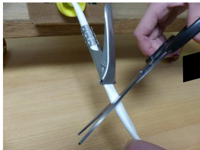
5 With the dispensing clip secured, snip the tap hose open.
